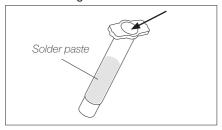
Fill in the syringe barrel with solder paste.
