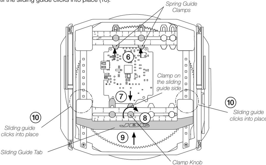
Now adjust the positions of the other sliding guide clamps to the PCB shape (11) and tighten their clamp knobs (12) after the adjustment.
