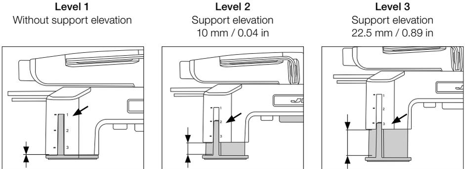
To adjust the height, press the two lower push tabs upward at the same time and hold them pressed (1).
