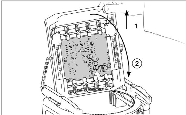
To do this, follow the same steps as for inclining the holder (1), but continue the tilting movement (2) until the PCB is completely turned over (3). If necessary, set again an inclined position using the positioning levers and arms.
