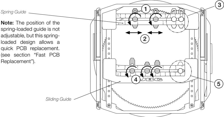
**Note:** The position of the spring-loaded guide is not adjustable, but this spring-loaded design allows a quick PCB replacement. (see section “Fast PCB Replacement”).
