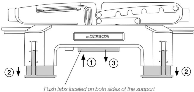
Lift the support while holding the tabs and let its feet drop down under their own weight (2).
