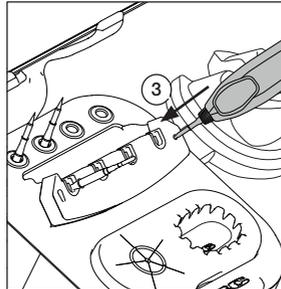
Gently press the tip against the holes on the sides of the cartridge exchanger (3) to ensure that the cartridge is appropriately inserted.
