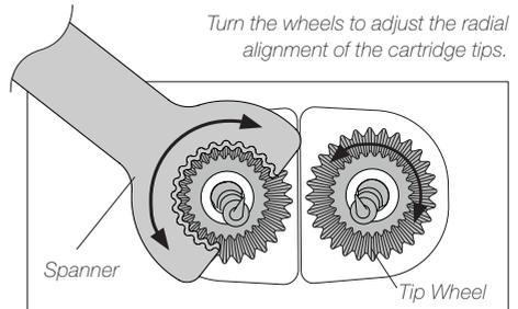
**Note:** The teeth of the spanner have the same inclination as the cone of the tip wheel. The spanner can be used from both sides, although it can only be inserted vertically.
