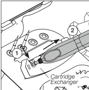
Place the tool over a cartridge and press the tool down to insert the cartridge (1). To release the tool with the cartridge inserted from the extractor, lift the tool upwards (2).
