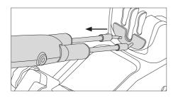
Insert the new cartridges using the cartridge exchanger. Then, press them against the thermo-resistant band to insert them completely\*.
