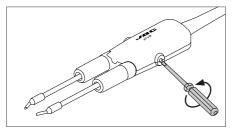
Unlock the fixing screws.
