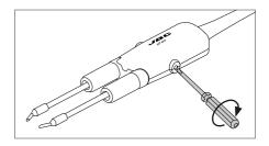
Lock the fixing screws.
