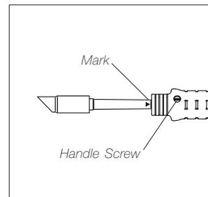
Make sure that the mark on the cartridge is aligned with the handle (see picture) to ensure a proper cartridge connection. Tighten the handle screw.
