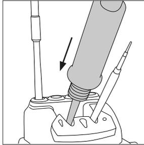
Place the handle on top of the new cartridge and press the handle down.
