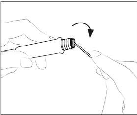
Introduce a small shaft or screwdriver, not deeper than 8 mm, and lift and pull out the sealing plug. Never use a cartridge to do this operation.
