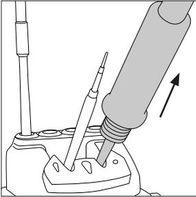
Place the cartridge in the extractor and pull the handle to remove it.
