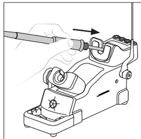
Place the handle on top of the new cartridge and press the handle down until the cartridge is fully seated.
