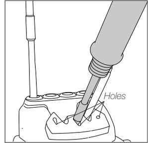
Depending on the shape of the tip, use one of the holes for fixing the cartridge.
