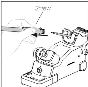
Loosen the handle screw. Place the soldering iron with the cartridge in the extractor and pull the handle to remove it.
