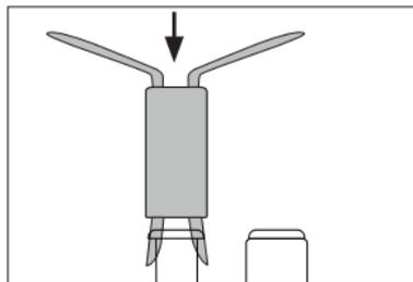
Push the grip with the fitters onto the tweezers.
