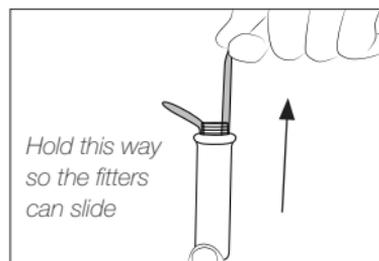
To remove the fitters, hold the grip and pull the fitters out. Use pliers if necessary.
