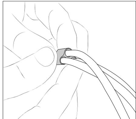
4. Use the tube clamps to hold all the tubes and cables so that they are more manageable and tidy.
