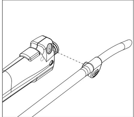
2. Assemble the suction nozzle and the clamp to the tool by matching the protrusion of the clamp with one of the side hollows of the tool (2).
