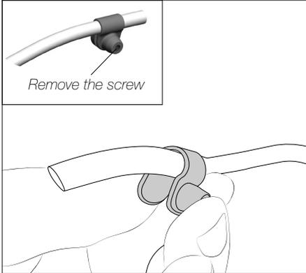
1. Unscrew the suction nozzle's clamp and take out the screw. Make sure that the nut and the suction nozzle stay in place.
