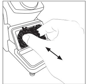
Replace the brass wool with a new one when it is worn out. Place the wiper back or replace them if desired.
