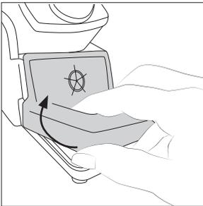
Lift the wiper at its front edge.
