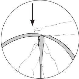
Insert the cable into the clip and then insert into the cable collector. Do not leave the cable longer than necessary to reach the work area freely.
