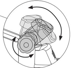
Adjust the tool holder angle to suit the work position.
