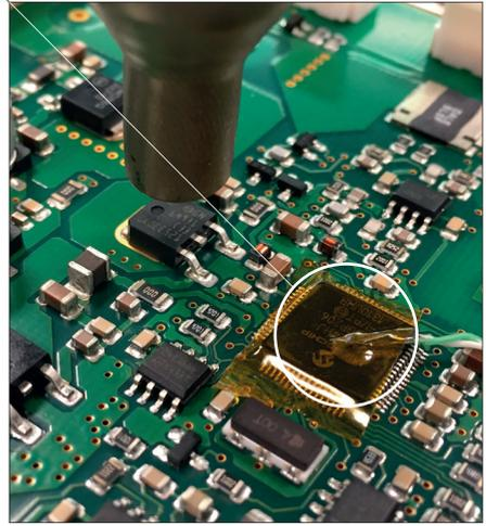
IPC\* does not recommend exceeding ramp-up rates over 3-4°C / sec. (5-7°F / sec) so as to reduce the risk of thermal stress on the PCB.
