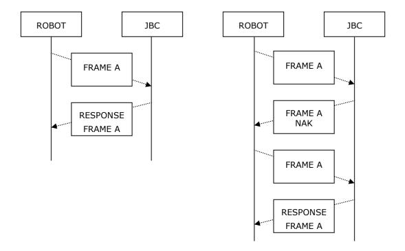
The number of repetitions followed by erroneous frames is determined by the Robot programmer.
