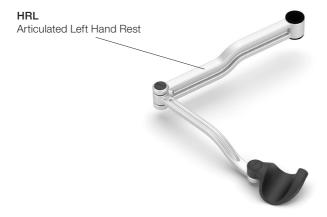
In the case of using both left and right arms, assemble both as shown in the illustration according to the letters on the back of the hand rest. To keep the hand supports at the same level, the right hand rest should be assembled below the left hand rest.
