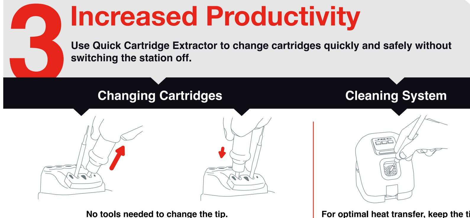
For optimal heat transfer, keep the tipeduces yourclean, tinned and thus free of oxides.
