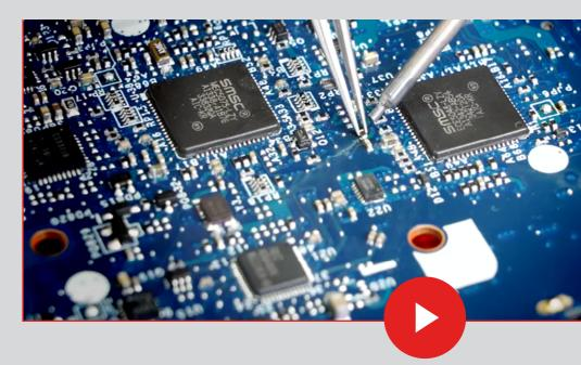
To enable operators to precisely position and remove ultra-miniature components, the JNASE Station includes a Pick and Place tool.
