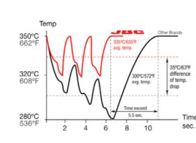
recover between connections, resulting in poor quality coldsoldered connections. To compensate for this, an operator will often run a conventional tip at a higher temperature. This can shorten the tip life and may even damage the PCB or the component being soldered - see graph.
