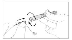
Thread the tip onto the syringe barrel.
