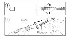
1. Note that the plunger goes into the syringe barrel with its head facing forward. Otherwise, DPM does not work properly.
