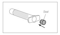
Take the barrel filled with solder paste and place the seal into the barrel.
