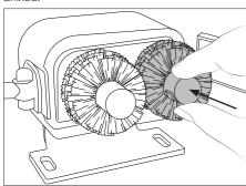
The Splashguard also works as a tin collector Clean it and place it back in its position.
