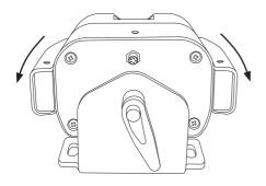
To pivot the CLMRP/CLMR, loosen and tighten the handle to turning it. The Handle can be aligned vertically again by pressing the Push Button.
