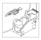
When the wire stripper is lifted from the stand, the cartridges will heat up according to the selected configuration.
