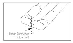
Align the tip edges and fix the cartridge in its working position.
