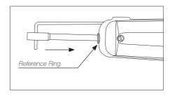
Insert the cartridge until the reference ring touches the wire stripper. Take the ring as a reference and check that both tips match.
