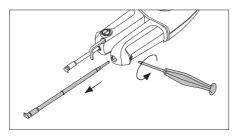
Loosen the screws and remove the cartridges.
