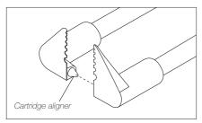
Align the cartridges in working position using a flat pliers (JBC Ref. PLR-195).
