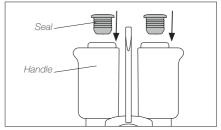
**Note** the sealing plug mounting position: The chamfered side has to be positioned towards the handle.
