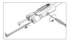
Loosen the screws and remove the cartridges.
