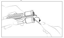
Enter a small shaft or screwdriver in order to gently lift and pull the sealing plug.
