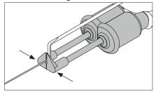
Choose cartridges according to the wire diameter. Pinch the wire with the blades. The pinched area will be melted by heat.
