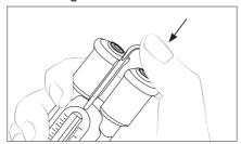
Gently push the sealing plug inside the handle until it is completely into the handle. Handle and seal edges have to be aligned.
