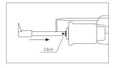
Insert the cartridge until the reference mark. Take the mark as reference and check that both tips match.
