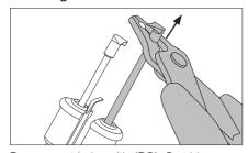
Remove cartrigdes with JBC's Cartridge Extractor Pliers (Ref. PLR195).
