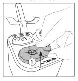
Assemble the new wiper membrane in vertical direction
