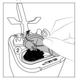
Press it down and make sure that the wiper membrane is correctly inserted all around (4).
