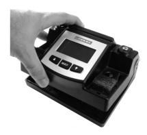
Place the housing back on without screwing it.
