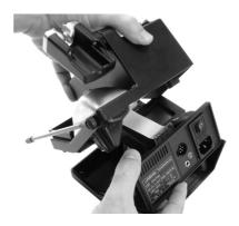
Place the lid back on without screwing it. Plug the power cord.
