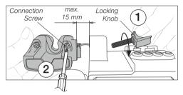
Using a flat-blade screwdriver, guide the cable connector outward to completely detach the support from the station. Any force exerted for extraction must be applied on the connector, never on the cable.
