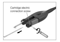
**WARNING:** It is essential to tighten the screws for the tool to function.
