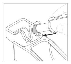
Attach the nozzle and press the nozzle onto the heating element with the help of the opening in the nozzle exchanger.
