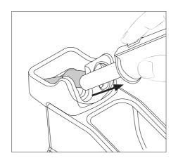
Place the heating element with the assembled nozzle in the nozzle exchanger and pull the tool to remove the nozzle.
