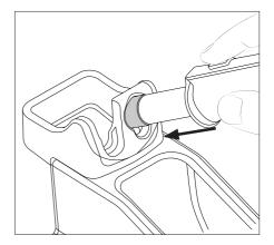
Attach the nozzle and press the nozzle onto the heating element with the help of the opening in the nozzle changer.
