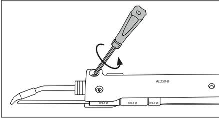
Unlock the cartridge fixing screw.
