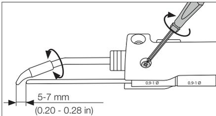
Align the cartridge tip with the solder guide tube. Leave a gap of 5-7 mm (0.20 - 0.28 in) between the tip and the end of the guide tube.
