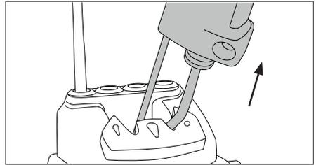
Place the cartridge in the extractor and pull the tool to remove the cartridge.
