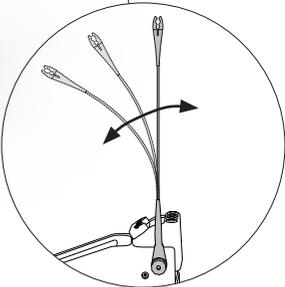
The Cable Collector is flexible. It accompanies and adapts to the movements during the soldering process.
