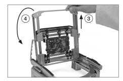
The holder is now completely turned around by 180° and the top side of the PCB is facing down (5).
