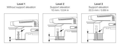
To adjust the height, press the two lower push tabs upward at the same time and hold them pressed (1).
