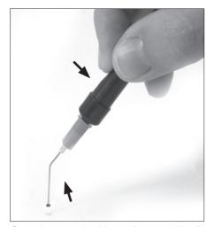
Cover the pen hole with your finger and lift off the component.
