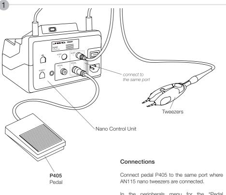
In the peripherals menu for the "Pedal Activation Mode" choose between "pressed" and "released".
