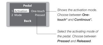
\* One-touch activates the pedal function until pressed twice. Continous activates the pedal function while pressing the pedal.
