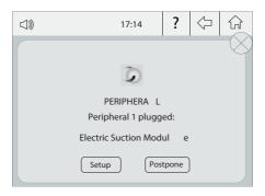
**2.** Select the module from the list of peripheral connections. Remember your first connection is denoted as "a", the second being "b", etc. (e.g. MS\_a, MS\_b,...). Do the same with the pedal (e.g. PD\_a,...)
