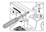
Reassemble the tool holder (3) and fasten the locking screw with the Allen key (1).
