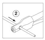
Insert the tool holder (2) by its bottom side through the connection.
