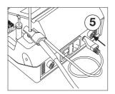
Plug in the pedal connector (5) to the equipotential connector at the back side of the station.
