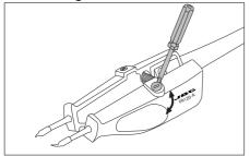
Unlock the fixing screws.
