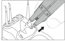
Place the cartridges in the extractor and pull the tweezers to remove the cartridge.
