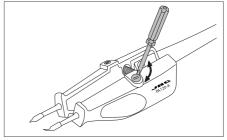
Lock the fixing screws.
