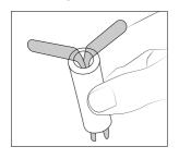
Insert the slide-on tabs into the new grip.
