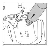
Place the cartridge in the extractor and pull the handle to remove it. Use the ring (J325) or umbrella (J125) around the cartridge as a stop to extract it from the tool.
