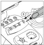
Gently press the tip against the holes on the sides of the cartridge exchanger (3) to ensure that the cartridge is appropriately inserted.
