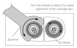
Note: The teeth of the spanner have the same inclination as the cone of the tip wheel. The spanner can be used from both sides, although it can only be inserted vertically.
