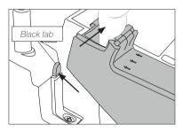
2. Separate both parts of the cleaning system to remove the brush.
