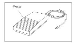
Press the Pedal P405 to blow hot air and release it to stop.
