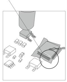
IPC\* does not recommend exceeding ramp-up rates over 3-4  $^{\circ}$ C / sec. (5-7  $^{\circ}$ F / sec) so as to reduce the risk of thermal stress on the PCB.
