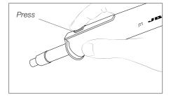
Press the start/stop button to blow hot air.
