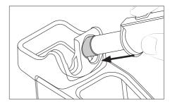
Attach the nozzle and press the nozzle onto the heating element with the help of the opening in the nozzle exchanger.
