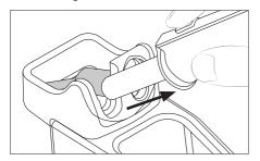
Place the heating element with its nozzle in the nozzle changer and pull the tool to remove it. The nozzle comes to rest in the nozzle holder.
