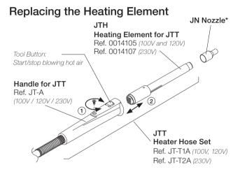
**Note:** Only perform this operation when the heating element is cold and the unit is disconnected from the mains.
