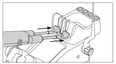
Remove the tweezers, press the tips against the cartridge exchanger and make sure that the cartridges are inserted correctly.
