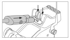
Once the previous cartridges are removed from the stand, insert the new cartridges into the two outer grooves. Position the tweezers over the cartridges and press it onto them.
