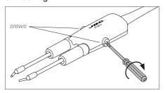
Finally lock both cartridge fixing screws.
