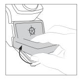
Lift the wiper at its front edge.
