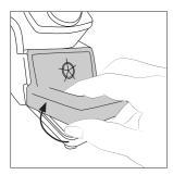
Lift the wiper at its front edge.
