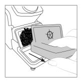
Remove the wiper by pulling it out.
