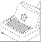
The softest cleaning method. Keep the sponge damp with distilled water when working to avoid tip wear.
