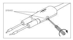
Lock the fixing screws.
