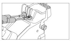
Use the grooves to insert the cartridges as far as the mark  $\!\!\!\!\!\!\!\!\!\!\!\!\!\!\!\!\!$  .
