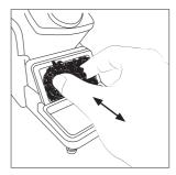
Replace the brass wool with a new one when it is worn out. Place the wiper back o replace them if desired.
