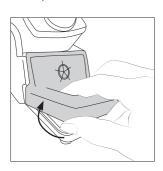
Lift the wiper at its front edge.
