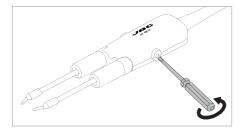
Unlock the fixing screws.
