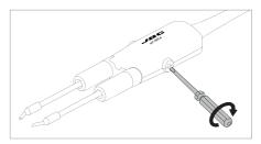
Lock the fixing screws.
