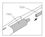
**3.** Insert a new filter (ref. 0008473) into the tool and mount the tube onto the filter.
