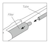
**2.** Remove the filter form the tool.
