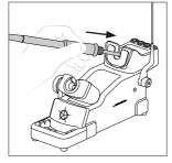
Place the handle on top of the new cartridge and press the handle down until the cartridge is fully seated.
