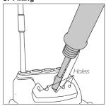
Depending on the shape of the tip, use one of the holes for fixing the cartridge.
