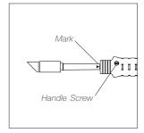
Make sure that the mark on the cartridge is aligned with the handle (see picture) to ensure a proper cartridge connection.
