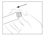
Push the sealing plug all the way into the tool.
