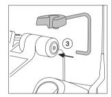
**Note:** The flat area on the tool holder bar must align with the threaded hole (4) on the back of the station.
