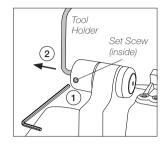
Insert the new tool holder bar into the slot on the station (3) in vertical position and as far as it will go.
