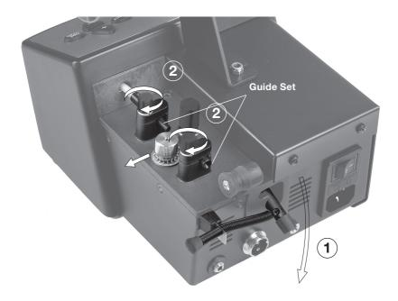
**3.** Insert the guide set in the tool. You must leave a gap of 8-10 mm between cartridge tip and the end of the guide tube.
