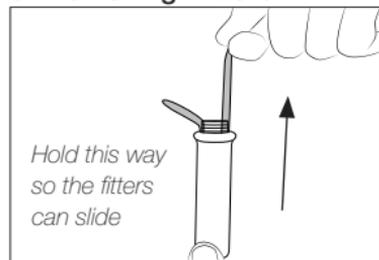
To remove the fitters, hold the grip and pull the fitters out. Use pliers if necessary.
