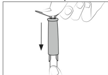
Push the grip with the fitters onto the handle.
