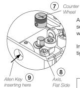
Assemble the counter wheel (7). Make sure that its thread entry for the set screw is aligned with the flat side of the axis (8). If not, the set screw will protrude, which may cause difficulties for the wire transportation.
