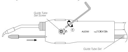
Unscrew the outlet nozzle. If the outlet nozzle is stuck onto the guide nozzle due to flux clogging, soak it in alcohol to release it.
