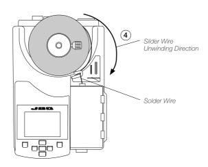
To assemble the reel locking, its conical side must be pointing downwards.
