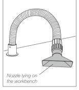
The nozzles are designed in such a way that they can be used with a hanging arm or be lying on the workbench
