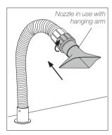
To install a new nozzle, align the bayonet, insert the new nozzle, and turn the nozzle clockwise to lock it in place.
