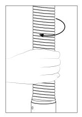
If the flexible arm loses firmness, it must be recompressed.
