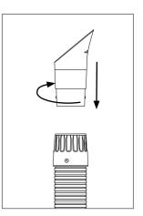
To install a new nozzle, turn the nozzle bayonet clockwise to lock it in place.
