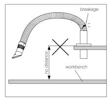
Do not install the flexible arm on shelves or higher levels than the work bench. Forced bending radii can cause the arm to break.
