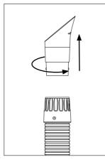
Disassemble the nozzle by holding the tube with one hand. With the other hand turn the nozzle counter-clockwise and pull it out.
