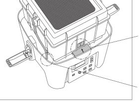
The filter has a given position. Make sure the filter ribs mate with the corresponding slots.
