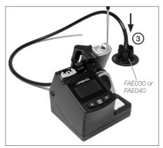
3 Connect the fume inlet duct for compact stations to the accessory for stand aspiration (Ref. FAE030 or FAE040), which should as well be connected to the fume extractor FAE through the hose FAE010.
